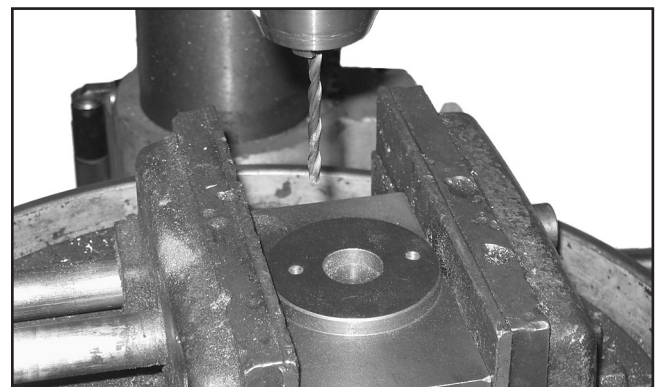
Figure 10. Guide pin holes drilled with 0.169" (or #18) drill bit.
