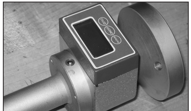
Figure 31. Large handwheel installed.
