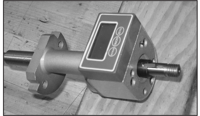
Figure 29. DRO attached to adapter shaft on leadscrew.
