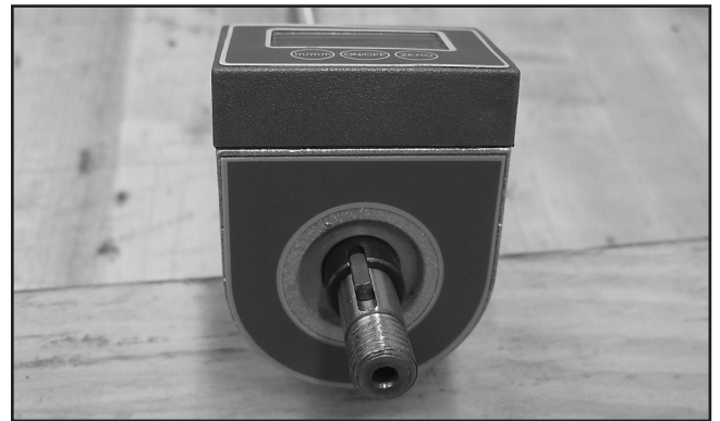
Figure 30. Beauty sticker placed on side of DRO to cover screw heads.
