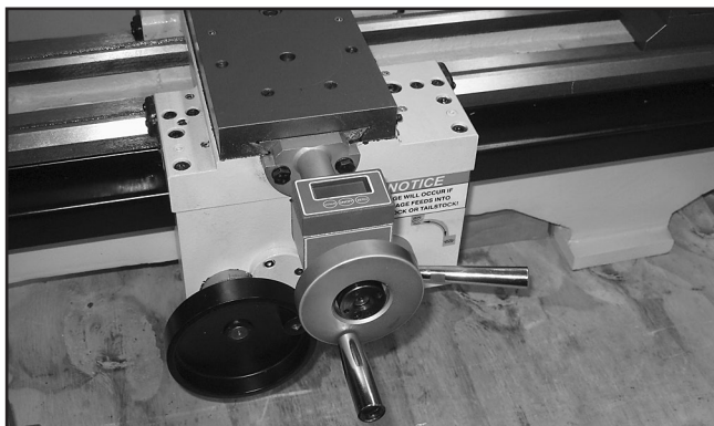
Figure 32. Cross slide DRO installed.
