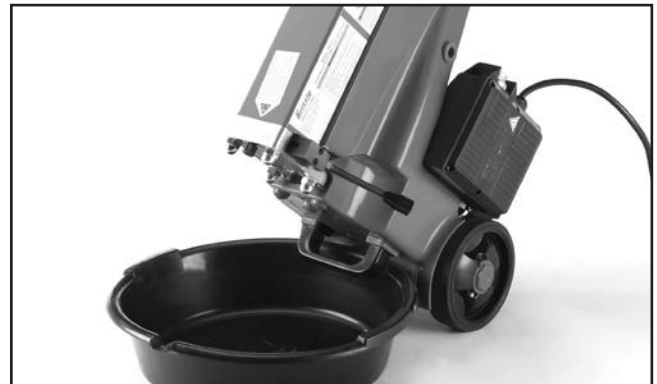
Figure 11. Draining hydraulic fluid.
