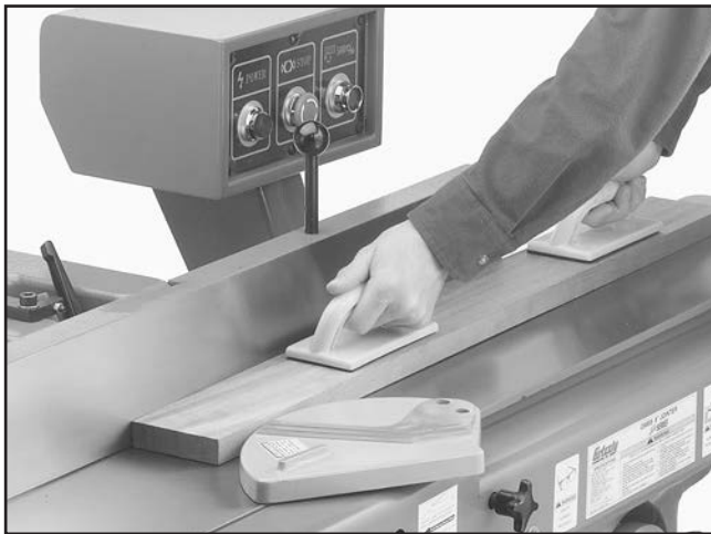
Figure 40. Example of surface planing with the jointer.
