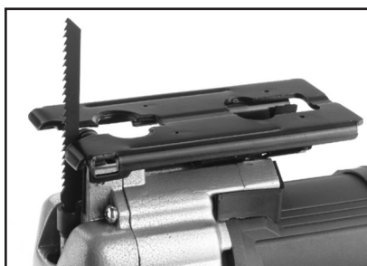
Figure 12. Footplate positioned for flush cutting.
