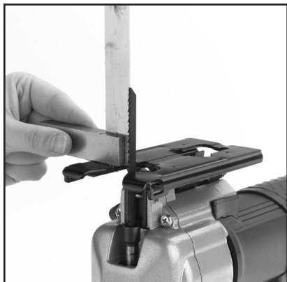
Figure 10. Checking blade squareness.
