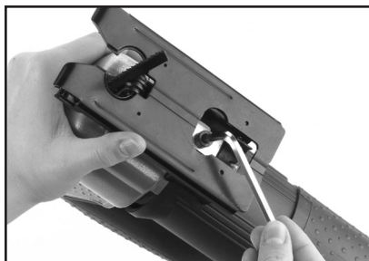
Figure 11. Setting footplate for angle cuts.
