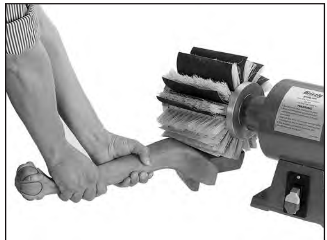
Figure 2. Typical flap sanding operation.
