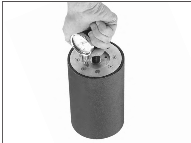
Figure 12. Checking sanding drum air pressure.
