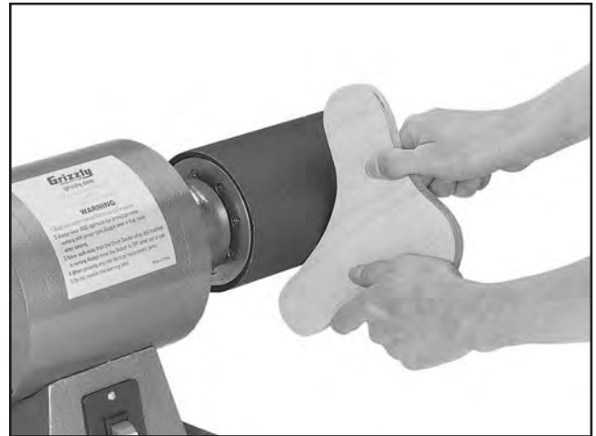
Figure 1. Typical drum sanding operation.
