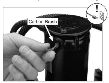
Figure 34. Carbon brush removal.
