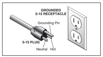
Figure 2. Typical 5-15 plug and receptacle.
