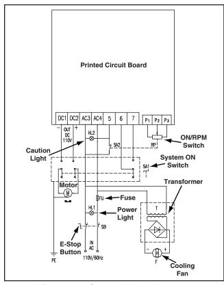
Figure 38. G8689 Wiring diagram.
