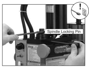
Figure 7. Loosening the drawbar.
