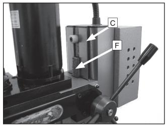
Figure 32. Upper column lubrication points.
