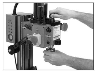
Figure 9. Removing the arbor.
