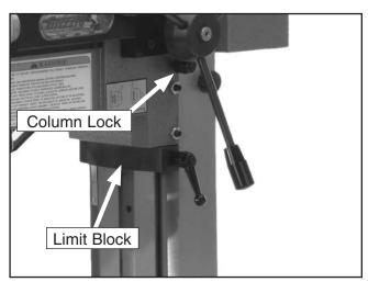
Figure 14. Limit block in place.
