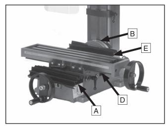
Figure 31. Points of lubrication.
