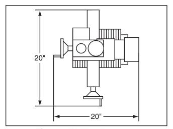
Figure 6. Working clearances.
