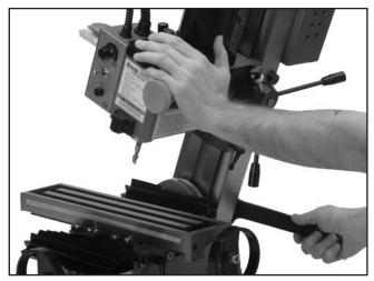
Figure 16. Supporting head during positioning.
