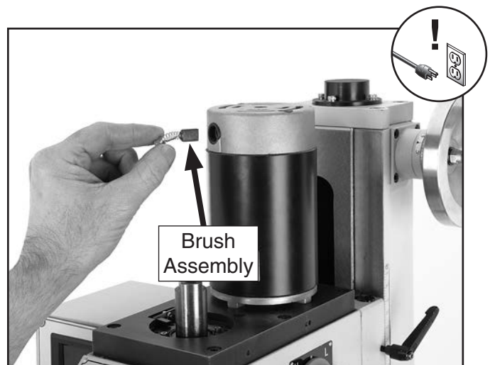
Figure 60. Installing new brush assembly.
