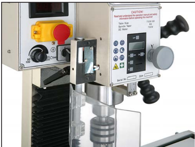
Figure 62. Chip guard limit switch.
