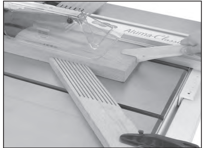
Figure 59. Typical ripping operation.
