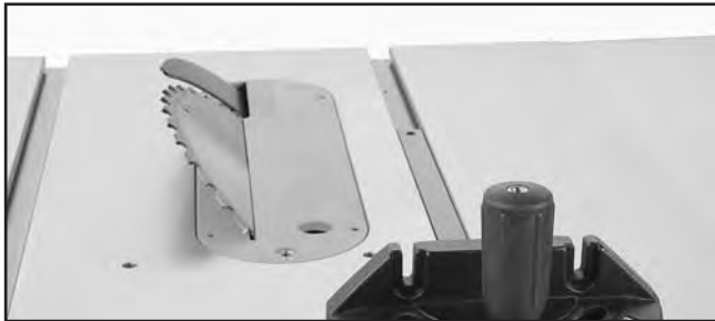
Figure 62. Blade tilted to 45° for bevel cutting on a typical table saw.
