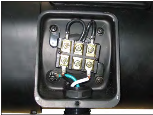
Figure 147. G0651 motor junction box.
