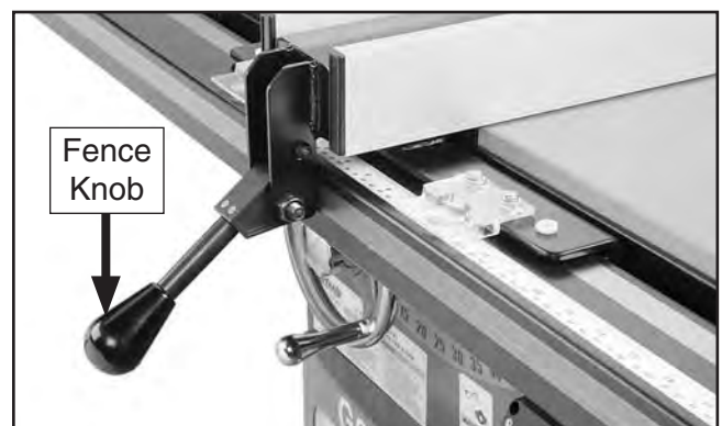
Figure 29. Fence knob installed.
