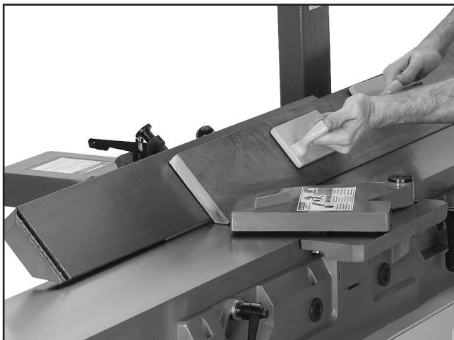
Figure 32. Typical bevel cutting operation.
