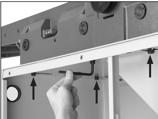
Figure 6. Securing jointer to stand.
