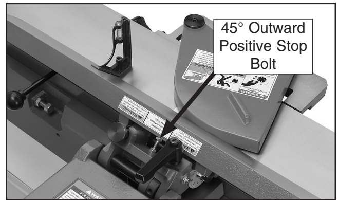
Figure 64. Adjusting fence 45° outward.
