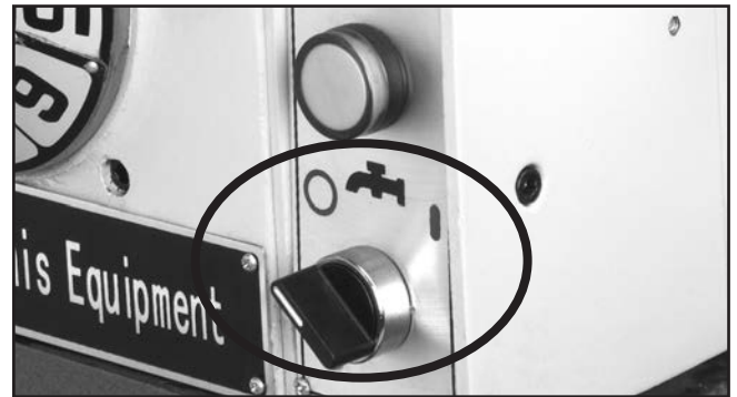
Figure 100. Coolant pump switch.
