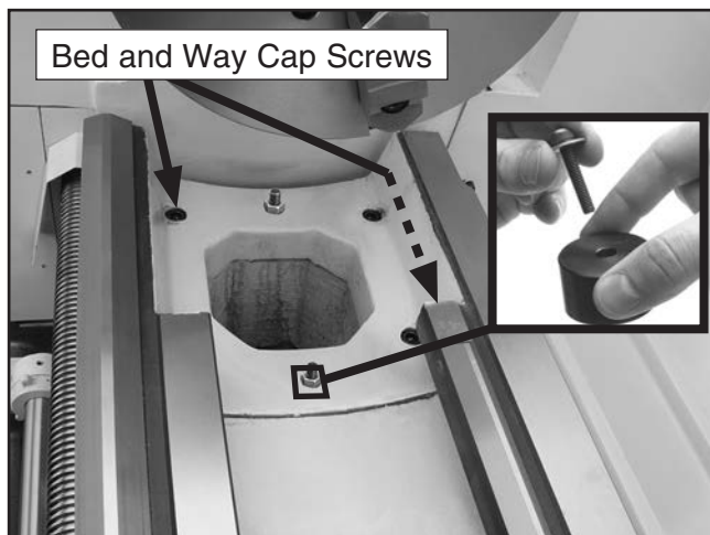
Figure 24. Lathe gap and pin puller setup.
