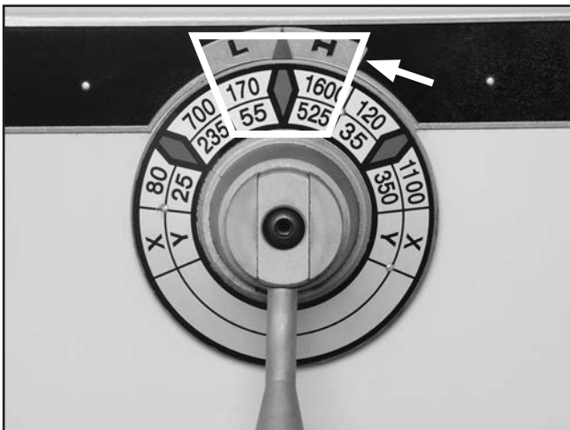
Figure 44. Spindle speed lever in central position—55, 170, 525,1600 RPMs available.
