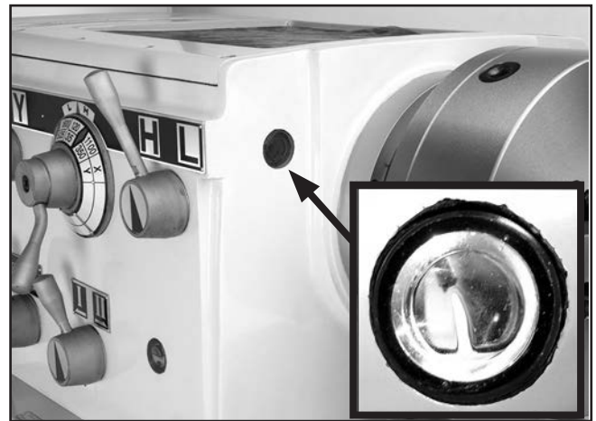
Figure 12. Oil pump sight glass.
