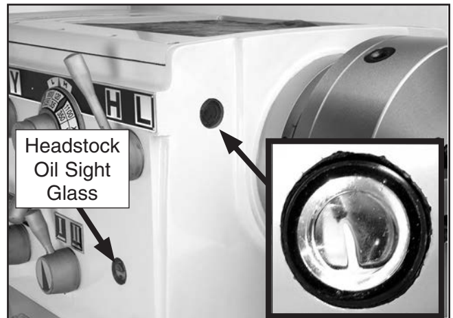
Figure 88. Oil pump sight glass.
