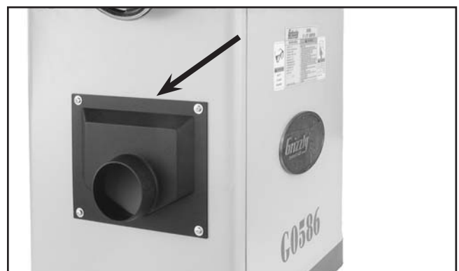
Figure 10. Correctly installed dust port.
