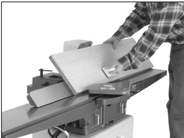
Figure 25. Typical bevel cutting operation.
