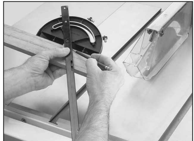
Figure 39. Marking miter line.
