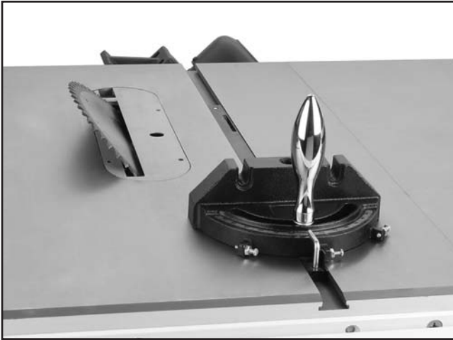
Figure 40. Blade tilted to 45° (guard removed for clarity).
