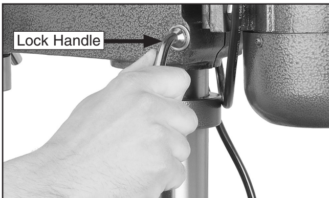
Figure 11. Securing headstock to column.
