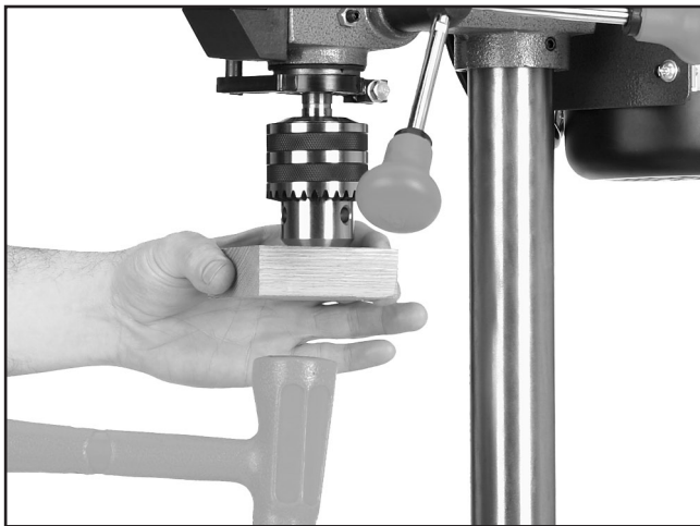
Figure 28. Seating the chuck on the arbor.
