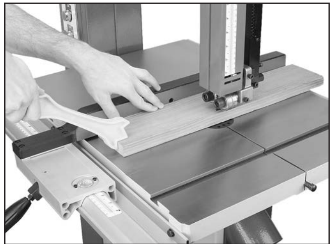
Figure 74. Ripping with a push stick.
