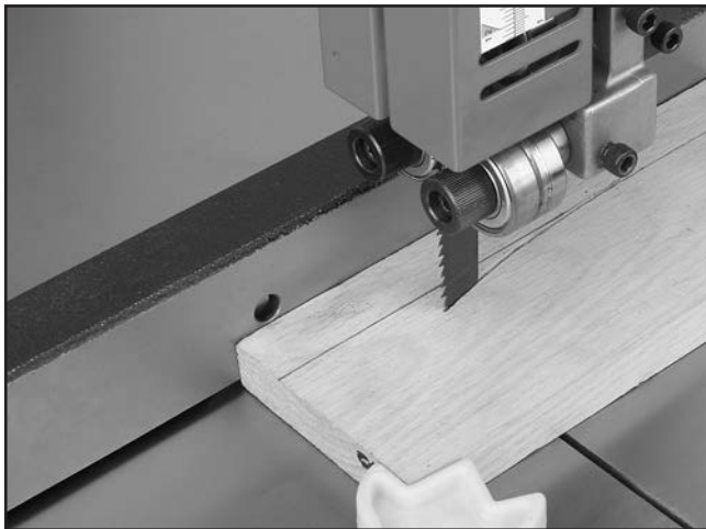
Figure 99. Blade leading away from line of cut.
