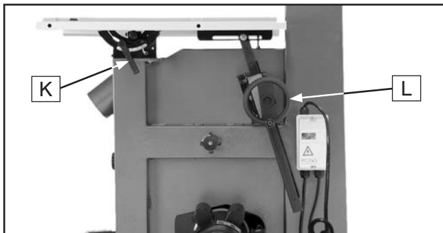
Figure 66. Table tilt controls (G0514X2, G0514X2B, and G0514X3)
