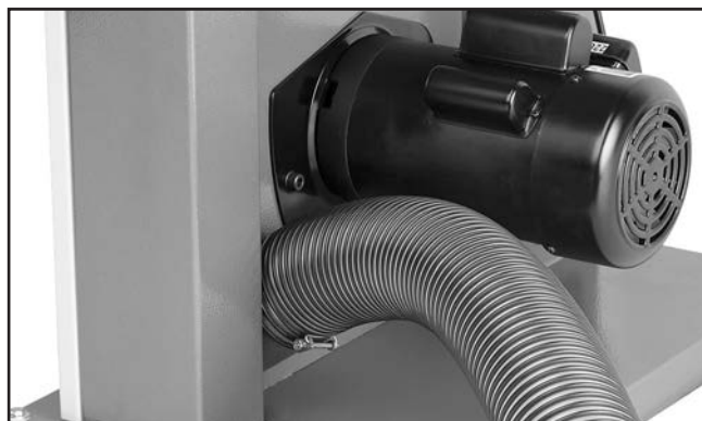
Figure 34. Dust hose attached to bottom dust port.
