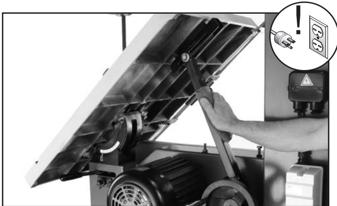
Figure 93. Example of lubricating table tilt rack and pinion assembly.
