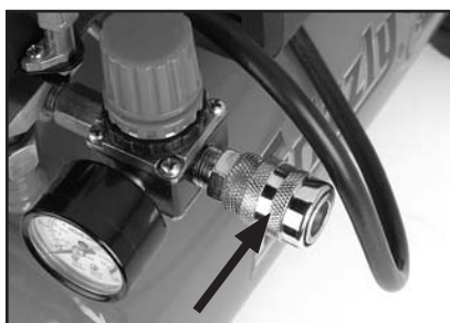
Figure 8. Quick connect coupler.
